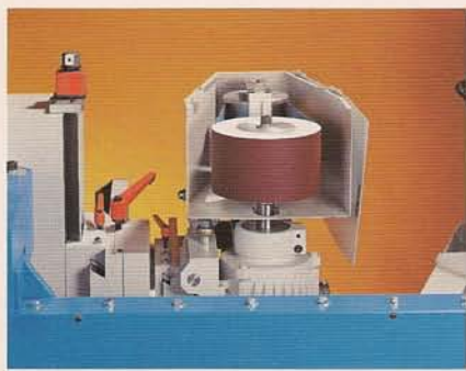
SPONGE WHEEL To supplement for sanding and grinding of the plain and curved surface.
