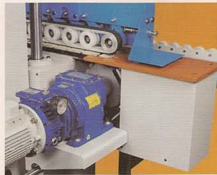
PRESSING • There are two kinds of press material : Roller type and Belt type. • The belt type is most suitably used for short and plywood workpieces.
