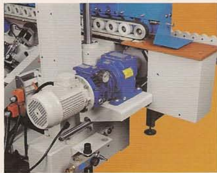
COVEYING The conveyor belt is transmitted with DISCO infinitely variable speed motor, and the conveying speed per minute is 3M~28M variable speed change.
