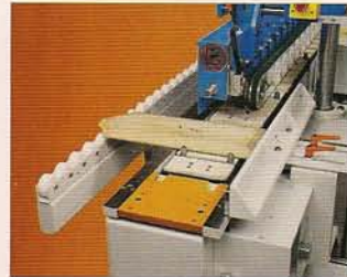
Conveyor 150m/m with stopper, hold down by single railed belt, feeding by inverter
