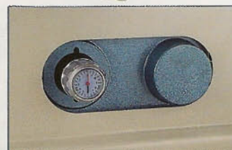
Variable feed speed change: range from 4-13 m/min
