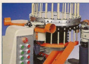
There are 24 guide tubes in a revolving tray.
