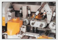
Side Front Pressure Plate on Left Vertical Spindle with Adjustable Table
