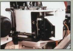
Vertical Spindle with Jointer Device (Optional) ~ for high speed feeding-60M / 80M / per min.
