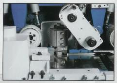
Vertical Spindle Adjustment up to 80 mm
