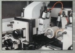
Pneumatic Cylinder for Chipbreaker on Top Spindle
