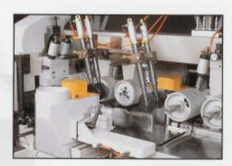
Extra Pneumatic Pressure Wheels for Vertical Spindle (Optional)
