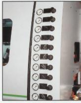
Individual Adjustable Pneumatic Pressure Gauges for Different Pneumatic Control Units
