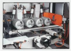
Powered Upper and Lower Feed Roller and Pneumatic Side Pressure Wheels
