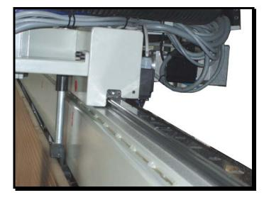
Hardened and ground *linear guides* for the vertical and horizontal feed, ensure smoothness without play
