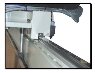
Hardened and ground *linear guides* for the vertical and horizontal feeds, secure smoothness in absence of play.
