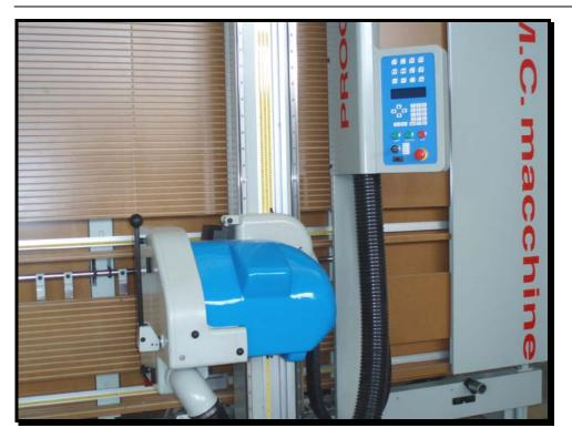
New compact and precise saw-group and control panel with electronic programmer for storing programs.
