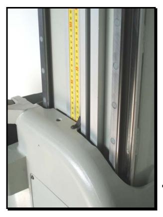
Hardened and ground *linear guides* for the vertical movement, secure smoothness in the absence of play.
