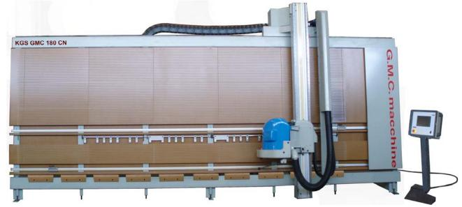
The main components of the frame machined on CNC machine tools allow dimensional accuracy during assembly, therefore, an excellent accuracy while using the machine. The movement on the vertical and horizontal axes, are ensured by hardened and ground linear guides, on which slide guide blocks that allow high sliding of the saw-head without play.
