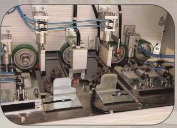
The PU rollers with high speed feeding, simple adjustment clamping unit secure the boards flat to the bed and square to the fence, guaranteeing a square, accurate cut every time.
