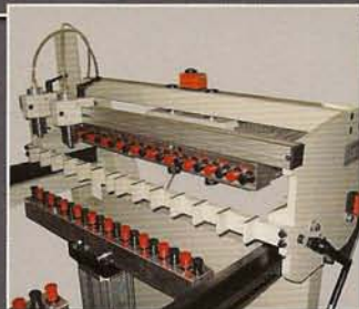
"Tilting horizontal boring unit" with 21-spindles and slides over the vertical boring units.
