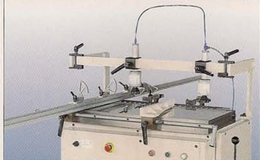
Optional: Long auxiliary aluminum fence(3M) & stoppers.
