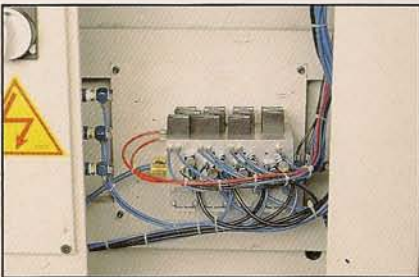
Pneumatic sequence controller: All pneumatic compounds are directly installed onto the integrated circuit distributor. Very easy change pneumatic parts.(Optional)
